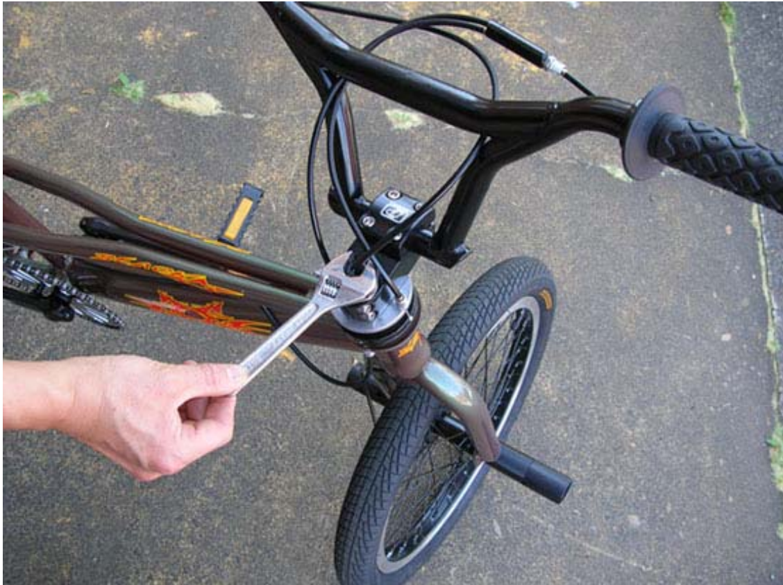
Now tighten the center bolt in the headstem, this will eliminate freeplay
