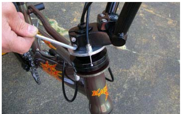
The side Allen key bolts should both still be really loose, so retighten them
