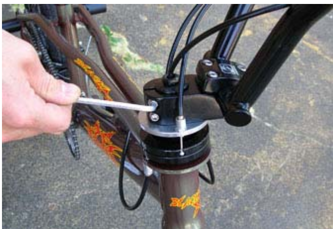
The side Allen key bolts should both still be really loose, so retighten them
