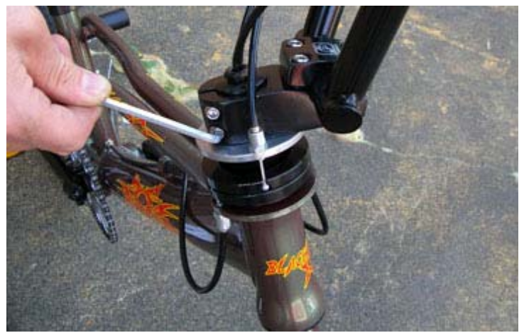
Loosen Bottom Allen Key Shown
